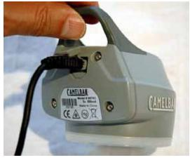
Once it's charged up, you're ready to go. Fully charged, it delivered twenty 60-second purification cycles before the battery level moved a notch, which was enough to convince me you could expect to be able to process more than 20 litres on a charge – enough for several days away from power. If you are planning a longer stint away from the grid, a solar charger might come in handy.
